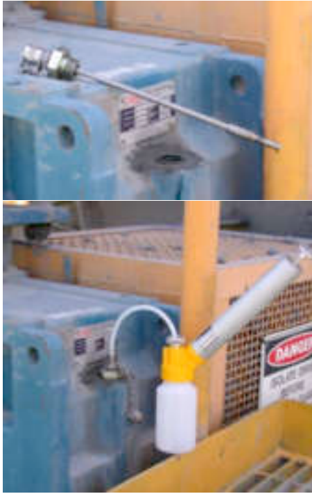
Examples of using a vampire pump in conjunction with permanent fittings, including a modified dipstick. (Ref: Pacific Power/PALL/Daryl Kelly)
