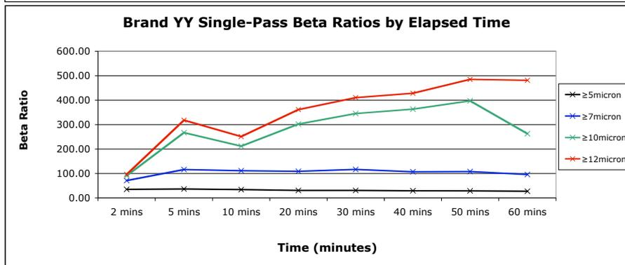
The elements from both manufacturers perform poorly at the target level of 2 micron. Neither element could be recommended in preference to the other.
