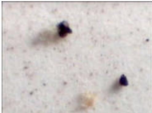
**This is a typical microphoto of diesel fuel. This sample was taken at the fuel bay post filter/coalescer at a mine site. (100ml of diesel, 47mm diameter membrane, 1.2 micron. Magnification 100x approx.**
