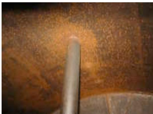
**Interior view of a horizontal diesel fuel tank. This is a picture of the ceiling showing large amounts of rust and corrosion that will further contaminate the diesel fuel. What is the more effective, reliable and proactive option? Paint the interior of the tank with a protective coating or rely on filtration?**
